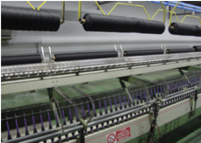
Yarn spinning (the slubbings are tensioned to make them thinner and twisted).
