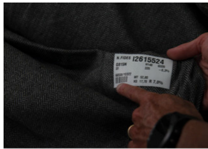
Barcode on fabric role for full traceability
