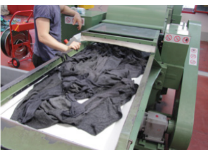
Knitted material ready for pulling
