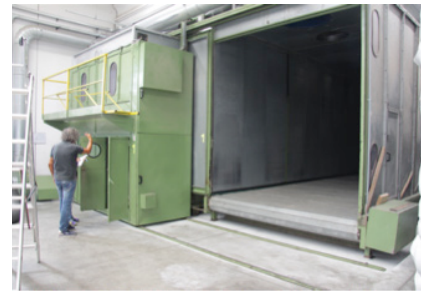
Container for blending (blending bin)
