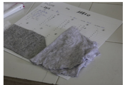
Colour control after washing and drying the felted sample. Result: sample is far too light in colour.
