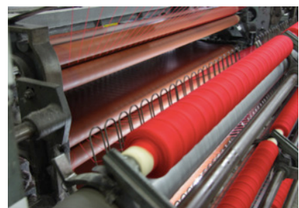
In-feed to the second carding section
